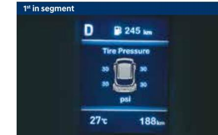
Tyre pressure monitoring system (TPMS) - highline
